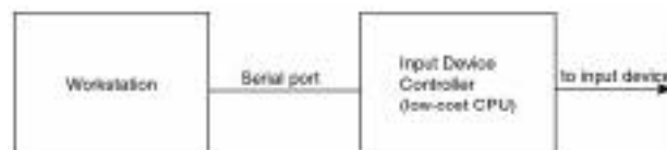
Figure 6-2 Input device connections to the workstation
