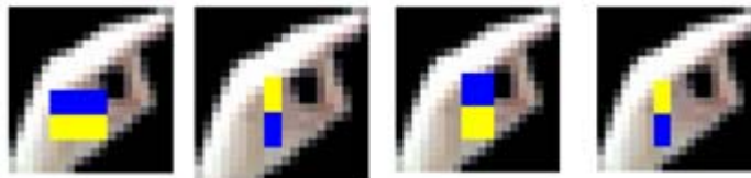
Figure 13. Four features selected by AdaBoost in the last stage. Features are shown overlayed on a typical training gesture. The features measures the difference in intensity between the region of the palm and the far side face of the hand.
