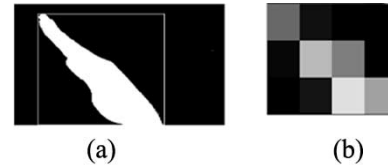
Fig. 2. Illustration of a feature extraction: (a) hand gesture within bounding box and (b) 3 \times 4 block partition.
