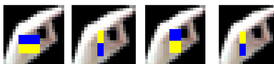
Figure 13. The four features selected by AdaBoost in the last stage. The features are shown overlaid on a typical training gesture. The features measures the difference in intensity between the region of the palm and the far side face of the hand
